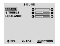
\* If neither the ◀ or ► button is pressed within 5 seconds, the current selection is set and the previous screen reappears. *To continue adjusting the sound* ... Repeat from step 2.
